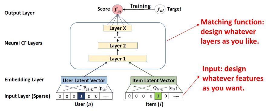
**Figure 2: Neural collaborative filtering framework**
